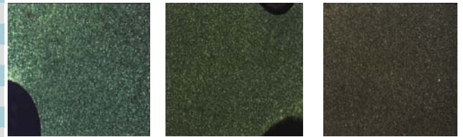
Fig. 2: Morphology for all the samples during isothermic crystallization at 160 °C
